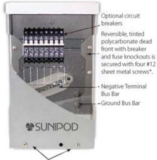
Two #12 sheet metal screws* secure the combiner's front cover.
